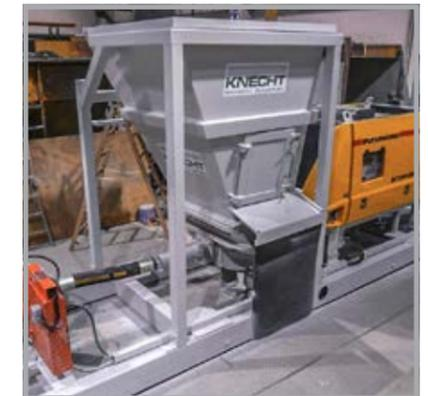
The buffer storage can be placed directly under the mixing plant or can be filled via an existing bucket conveyor.
