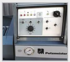
Operation of the machine directly from the control panel or via radio remote control
