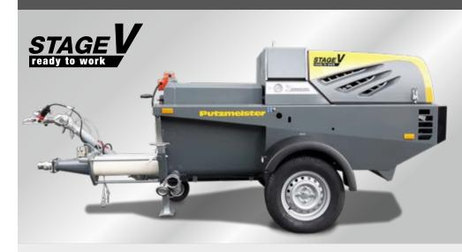
The SP 20 GHF is a worm pump for self-levelling floor screed applications. Equipped with a 4 cyl. Kubota 33 kW gasoline engine compliant with Stage V emission standard, this machine is very powerful and allows high delivery distances.
