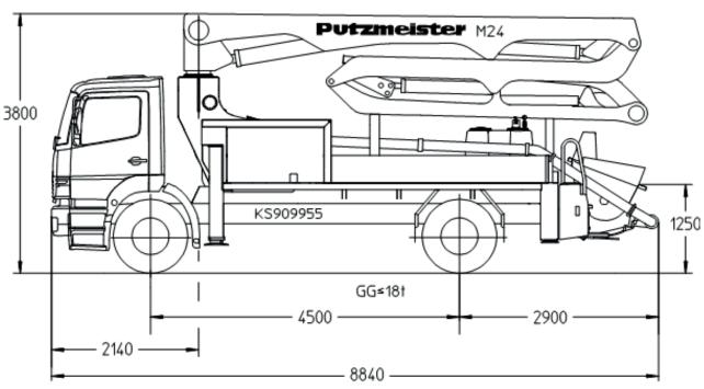
Note: Standard version.for .09 H and .11 H (LS). Dimensions and weights depend on truck, pump model and equipment. Dimensions in mm, MB-Axor 1828 as example.
