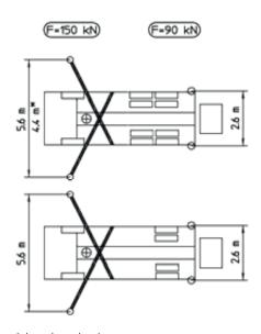
\* depends on chassis Dimensions can differ depending on configuration.
