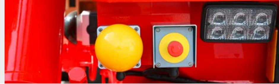
Additionally, Emergency Stop on the left. The driver can react quickly, he does not have to run forward to the support foot control or run around the mixer.
