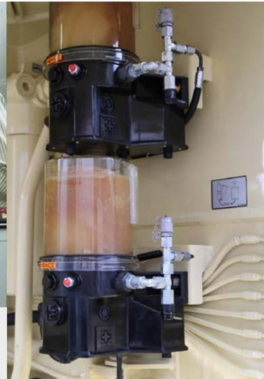
Automatic central grease lubrication system: The electrical central grease lubrication for the hopper ensures that the service life of the highly stressed components is maximized without any additional work.
