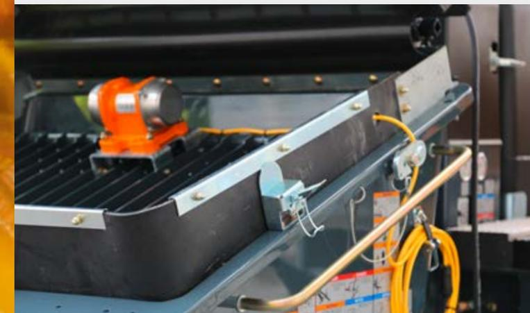
**Agitator safety shutdown via RFID** (Radio Frequency Identification): the detection system provides the help of electromagnetic waves, including start-up maximum safety for operators.
