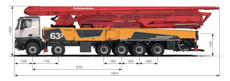
Note: Serial version. Dimensions and weights depend on truck, pump model and equipment. Dimensions in mm, MB-Arocs 6553 12x4 R6750 E6 as example For illustration only.
