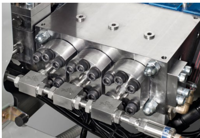
More power and safety: ultrahigh-pressure pump with full lift safety valve
